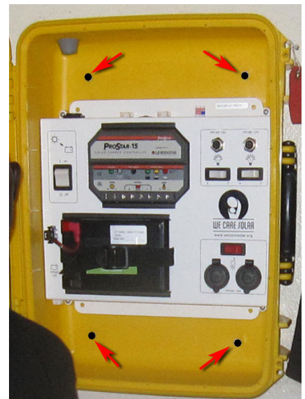
Be sure to drill the holes outside of where the main control board will go.
