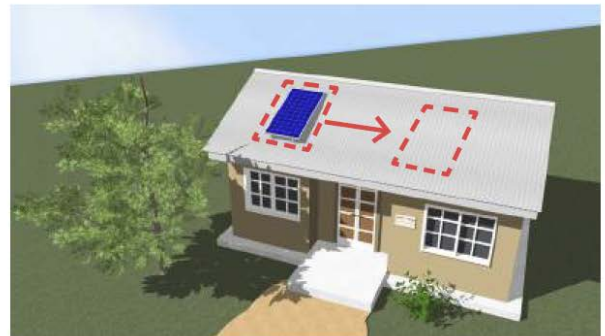
Trim the tree or move the solar panel to an area of the roof that is not shaded
