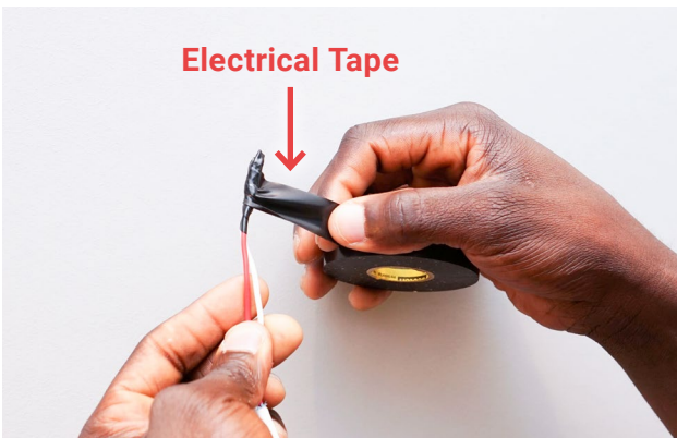
Wrap the ends of the wires separately with electrical tape to protect the wires
