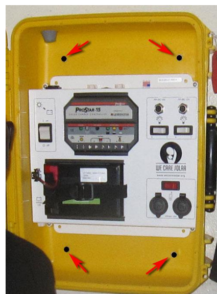
Be sure to drill the holes outside of where the main control board will go.
